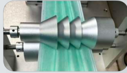
BOTH ENDS ULTRASONIC WELDING
