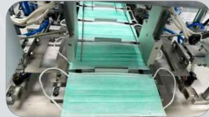
EAR LOOP ULTRASONIC WELDING
